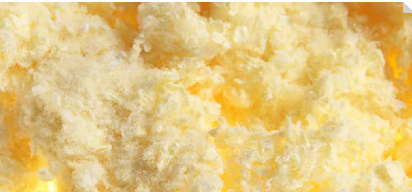
Cellulose Fibre Insulation (CFI) of recycled silicon-coated paper.
