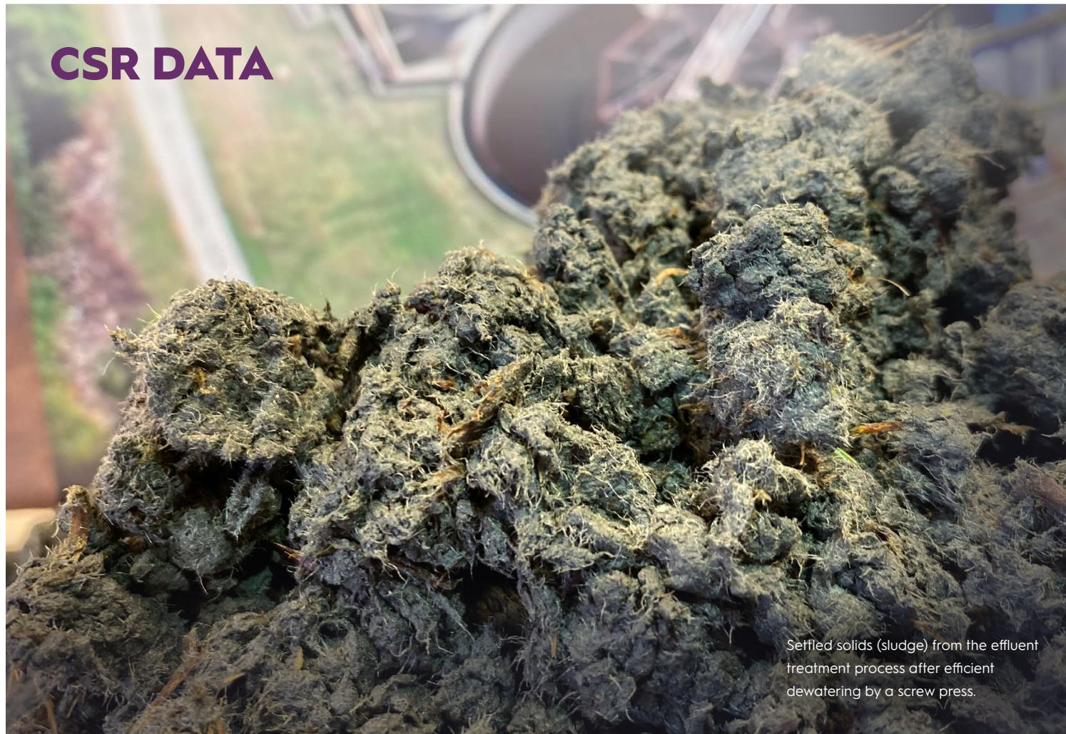
Settled solids (sludge) from the effluent treatment process after efficient dewatering by a screw press.
