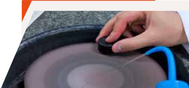
To prevent the slightest scratching of the specimen's surface, the choice of abrasives and their quality are crucial criteria that must be considered in advance. Fixed onto the polisher, the product selected will produce a mirror polish, or at least the finish required for the analysis. So:
