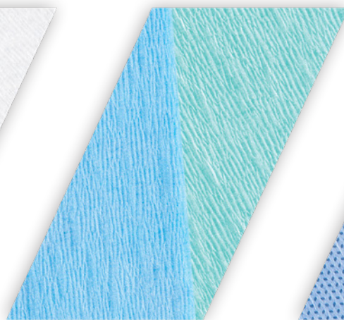
WETLAID NONWOVENS cellulose + synthetic fibers
