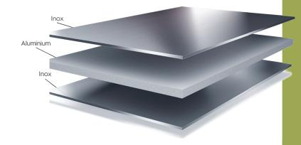
two layers of stainless steel. For that assembly to be perfect and the sheets to bond into one, it is necessary to prepare the surfaces before cladding by sanding them with abrasive paper. We also use it for final surfacing to give the products a slightly shiny polished finish, as you can see inside the grillplates you can buy in stores.
